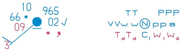
Figure 2. Sample station plot with plotting model. The left-hand plot shows a weather observation for Dublin Airport as it would be plotted on a weather chart; the right-hand plot shows the meanings of the various symbols. Thus, moving clockwise around the station plot (starting at the top right-hand corner) the symbols have the following meanings: 965 is the pressure (PPP); 02 the pressure change in the past 3 hours (pp) and the symbol beside this number indicates a fall in pressure followed by a rise (a); the full stop (rain) and the comma (drizzle) are codes for the weather during the six hours preceding the observation (W 1 , W 2 ); the horizontal line to the left of the past weather is the symbol for stratus cloud (C i ); the wind arrow indicates a wind speed of 10 knots coming from the south-west (230°) with the figure 3 indicating the second-last digit of the wind direction; 09 is the dew point (T d T d ); 66 a code for the visibility (VV); the full-stop to the right of the visibility is the present weather — rain (ww); 10 is the temperature (TT); and finally the station circle, at the centre of the plot, is shaded to indicate a cloud cover of 8/8 (N).
