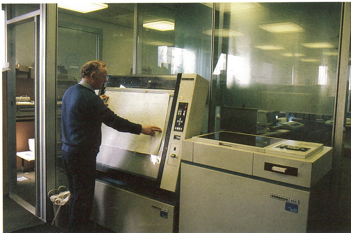
Removing a chart from the CALCOMP automatic plotter
