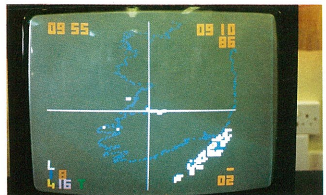
Precipitation off the south-east coast of Ireland shows up as a digitised radar image on a monitor screen at Shannon Airport.
