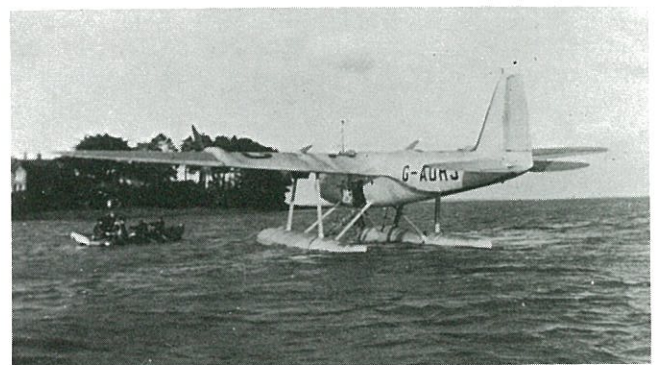
The 'Mercury' at Foynes, c. 1938/9. The 'Mercury' was the upper component of the 'Short-Mayo composite' — a 'pick-a-back' device consisting of two aircraft locked together for take-off. The lower aircraft, the 'Maia', provided the power needed for take-off up to a suitable height, when the 'Mercury' was released. The 'Maia' was destroyed in a bombing raid in 1941, and the 'Mercury' was broken up two months later. (Photo: F.E. Dixon)
