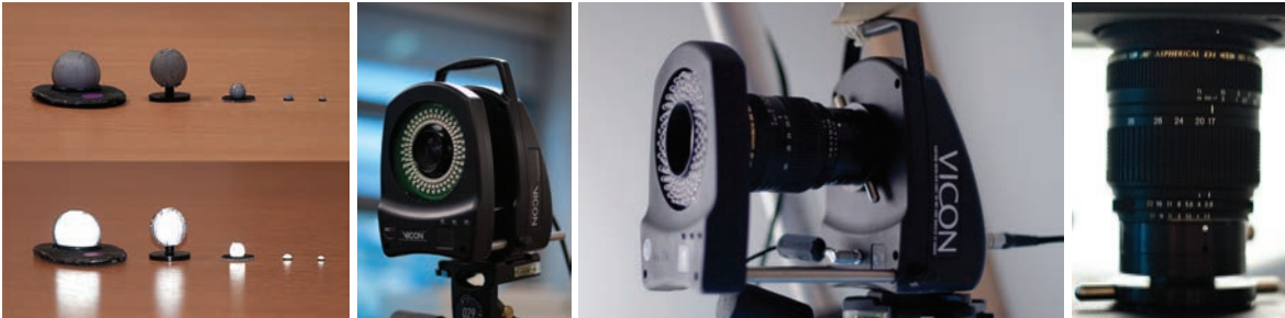
Figure 3.1.: Detailed view of our motion capture hardware. From left: Reflective markers used for motion capture, photographed without and with flash to demonstrate their back-reflective optical properties; a wide-angle IR camera; a narrow-angle IR camera; detail of a long-focal-distance lens with setup rings.
