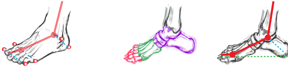
Figure 4.2.: The foot bones and their representation in our optical motion capture. Left – the relative location of the foot markers and its virtual bones; middle – an actual skeletal structure of the foot, with lower leg bones (black), tarsus (purple), metatarsal bones (green) and phalanges (red); right – side view demonstrating the implicit representation of the heel in the skeletal data.
