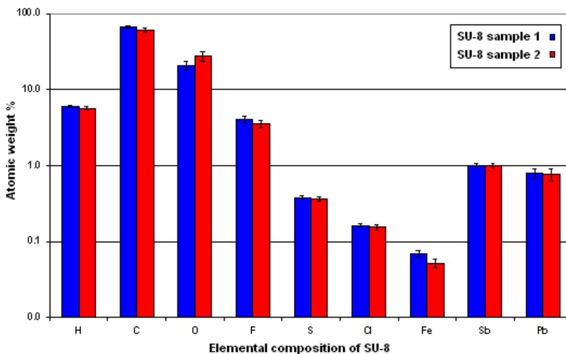
**Figure 1.3.** Atomic weight percentages of different elements in SU-8 samples 1 and 2, as determined by PGAA.
