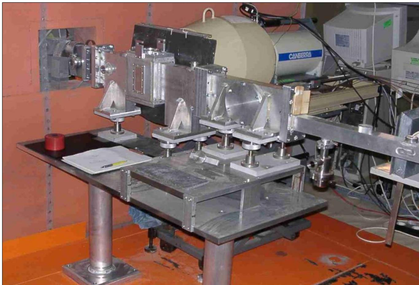
**Figure 1.1.** Prompt Gamma Activation Analysis station at the Institute of Isotopes, Budapest Research Reactor (BRR).
