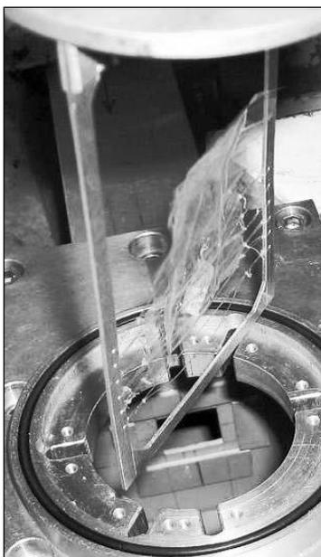
**Figure 1.2.** SU-8 microturbine sample fastened with Teflon strings onto an aluminium frame for introduction into the PGAA measurement chamber.
