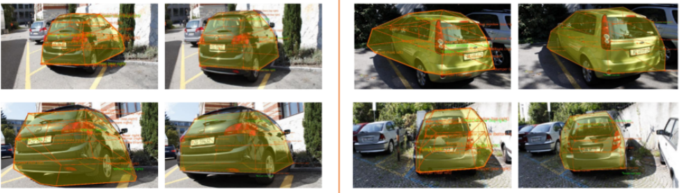
Fig. 8: An illustration on the improvement in Viewpoint and Shape Estimation due to the Viewpoint and Shape refinement step. Each pair of the image represents the Viewpoint and Shape estimations before ( left ) and after ( right ) the Viewpoint and Shape refinement step. The shapes on the right (of each pair) tend to be more compact and has a better viewpoint estimate, than the ones on the left.
