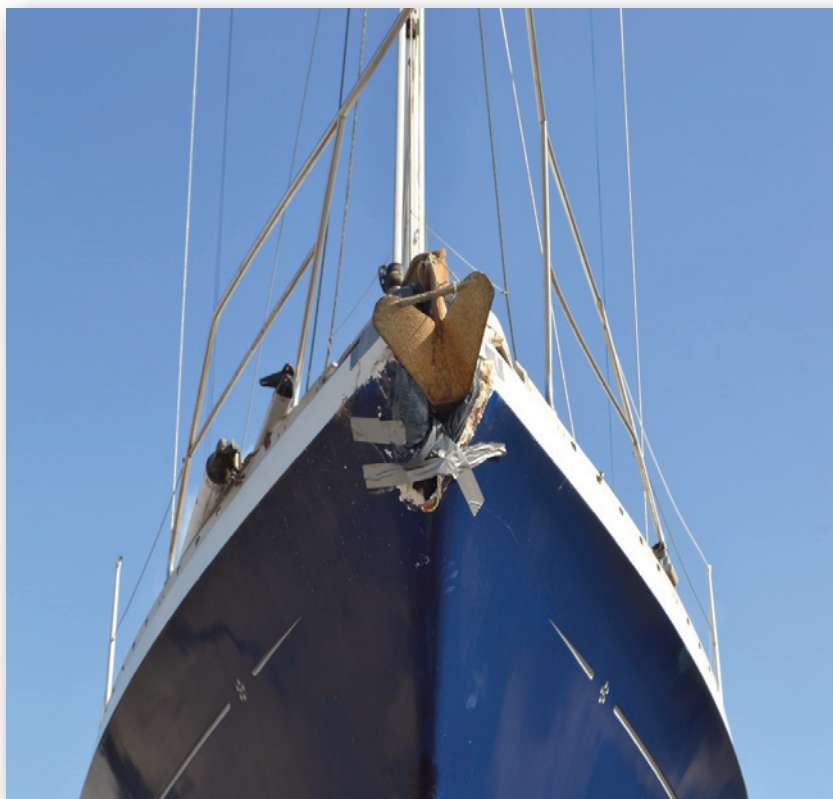
Photograph No.3 - Damage to bow of 'Medi Mode'.
