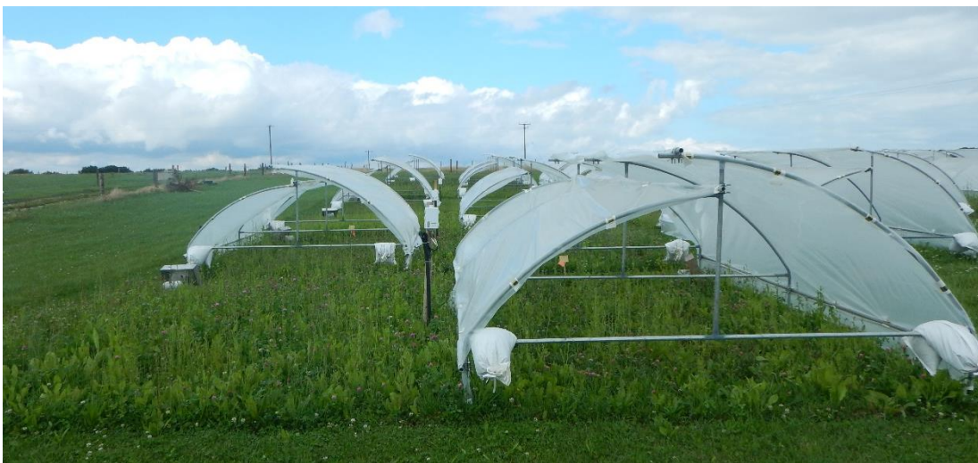
Figure S2.1. Photograph of the experiment. The front of the photograph shows a main plot with a six-species community sown, with the rainfed treatment on the left-hand side and the rainout shelter to simulate the drought treatment on the right-hand side.
