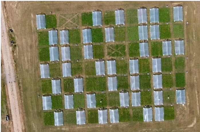
Figure S1.3. Drone picture of the experimental field in July 2018, with rainout shelters applied to one half of each plot. See Fig. S2.1 for a closer picture of a rainout shelter.
