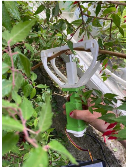
Figure 5.3: Portable three-point bending rig used in the field.
