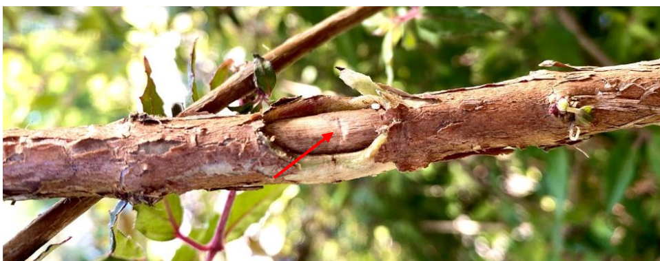
Figure 5.7: Specimen damaged and left to heal for 8 weeks. Callus has formed around the damaged area. Red arrow pointing to small amounts of compressive damage where the support pressed on the specimen during bending.
