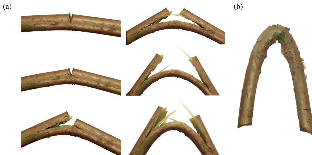
Figure 4.6:(a) Progression of greenstick failure in fuchsia. (b) Plastic hinge failure mechanism in fuchsia.
