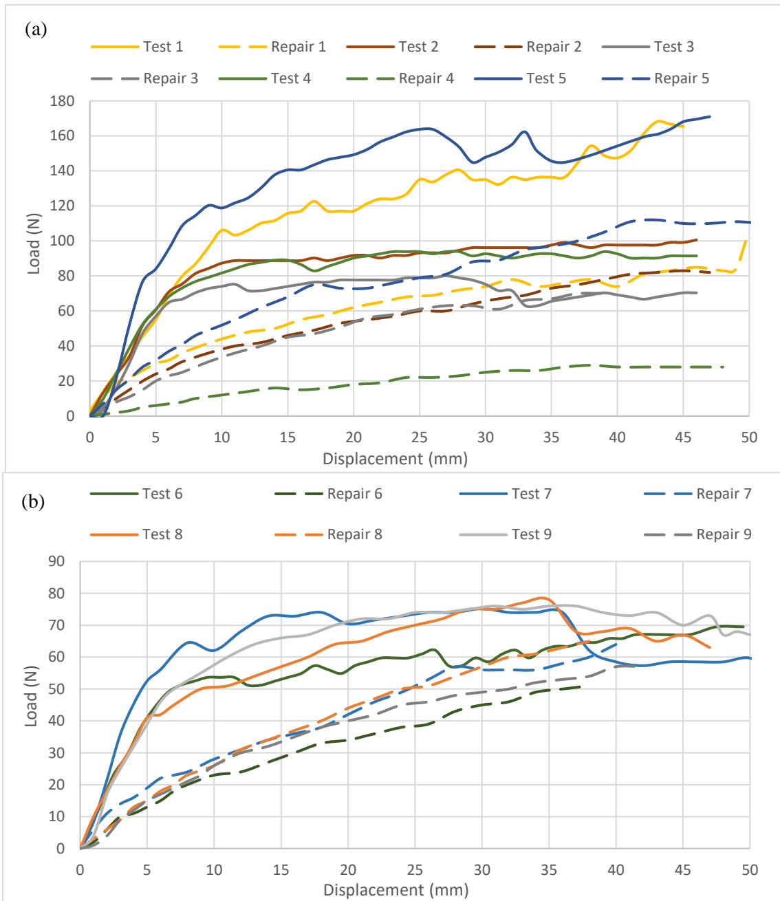
Figure 5.11: Effective load displacement curves adjusted from FEA correction factors on specimens left for 4 weeks to repair for (a) samples 1-5 and (b) samples 6-9
