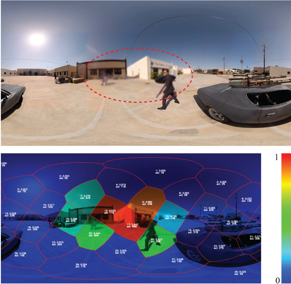
Figure 3.7: Example of sharpness mismatch score visualization: left ODI with blur inside the red ellipse (top) and sharpness mismatch visualization (bottom) including a text overlay with the sharpness mismatch patch score and the visual attention.
