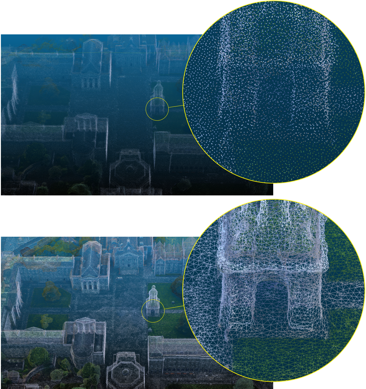
Figure 2.5: The first figure shows the point cloud data does not have connections between the points. The bottom mesh data shows the connections between the points. The point cloud data and mesh are generated by Pixel 4D with input aerial images from the Trinity drone dataset [28].
