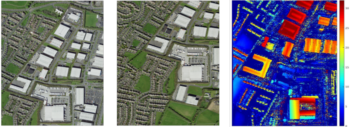
Figure 2.7: The disparity map (right) is generated from the pair of RGB aerial imagery. The dataset is provided by OSM [83].
