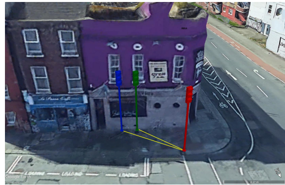
Figure 5.6: The left figure shows the positive ray intersection between the two. The red dot stands for ground truth position. The blue pairs are the camera pose with no correction, and the green pairs are the camera pose with correction. Their pair of rays intersect at the position with the same colour corresponding to their camera. As can be seen, the intersection of the green dot is closer to the ground truth. The right figure shows the position of intersection and ground truth in Google Earth in the same colour scheme.
