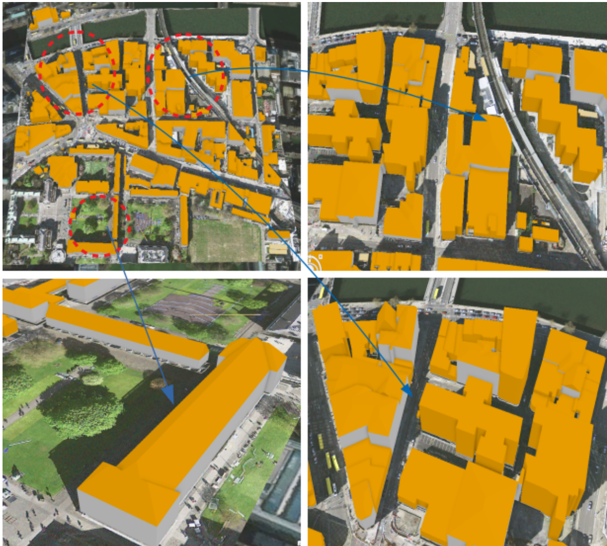
Figure 4.15: IM2ELEVATION inference results applied to roof profile estimation (LoD2).
