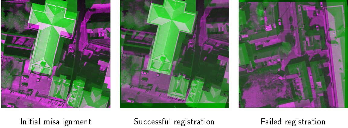
Figure 4.5: MI registration between return-pulse intensities (green) and optical image (purple) may fail when the scene content is significantly different between the two data sets.
