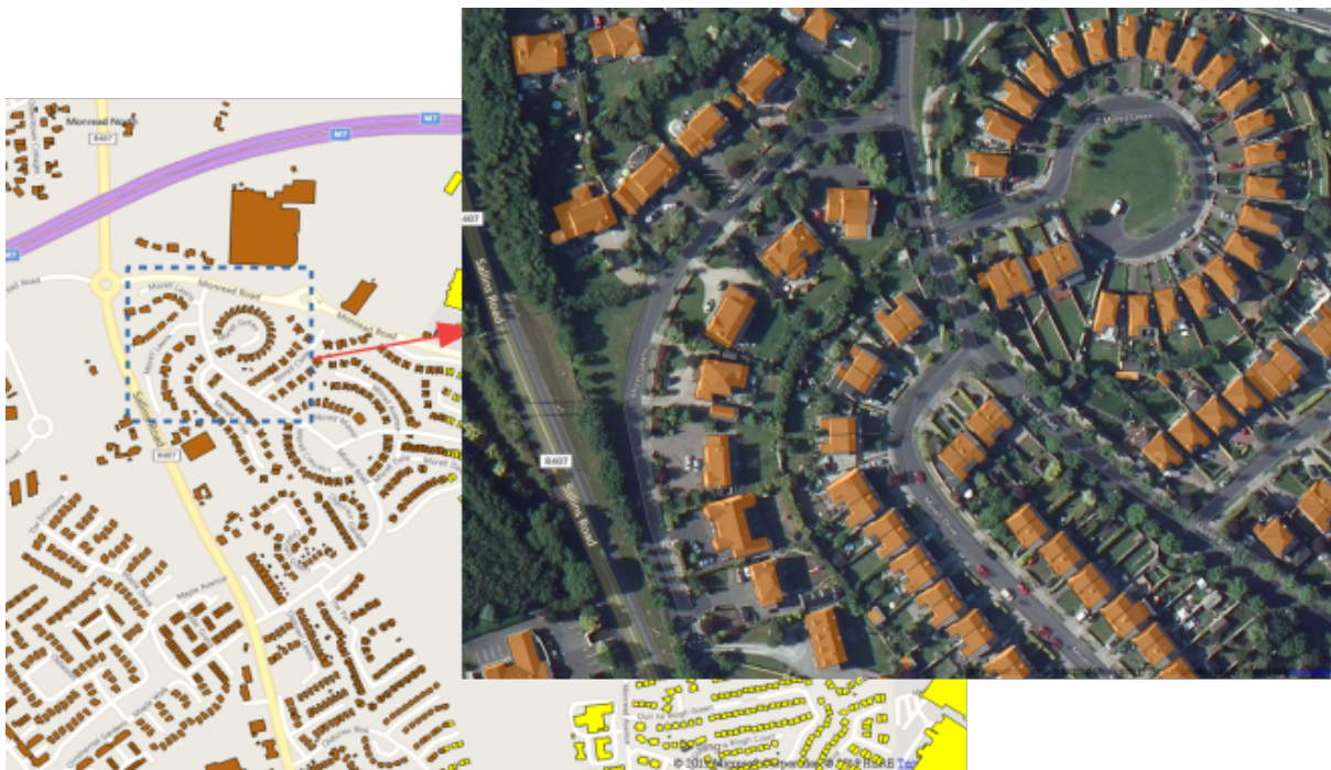
Figure 2.9: Overlay the building footprint from OSI map data [83] onto aerial image. The preparation of data can be used for supervised machine learning.
