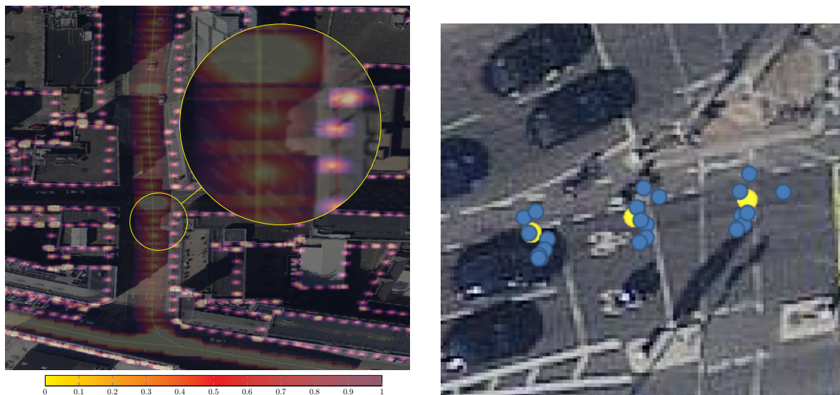
Figure 5.5: The figure (left) shows the prior map information overlaid on an aerial image. The normal kernel is applied to each node that is imported from OSM. The heatmap outlines improbable object locations that will have a smaller contribution to the weighted sum. On the (right) yellow dots are the positions taken from image metadata, and the blue dots represent their corrected versions with SfM.
