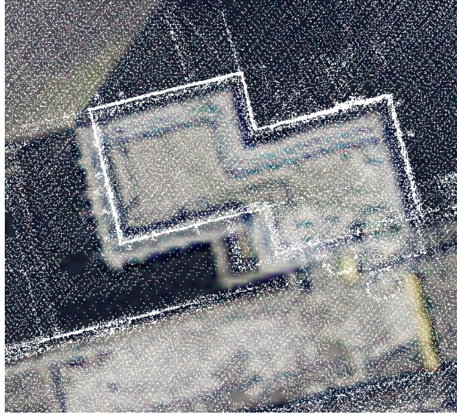
Figure 2.11: The misalignment can be seen from projecting 3D point cloud [75] onto the corresponding image [83] in the same georeference.
