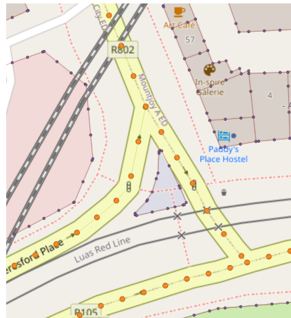
Figure 2.8: The data is imported from OSM. The nodes around the building (purple) form a polygon representing building shapes. The nodes in orange represent the road.
