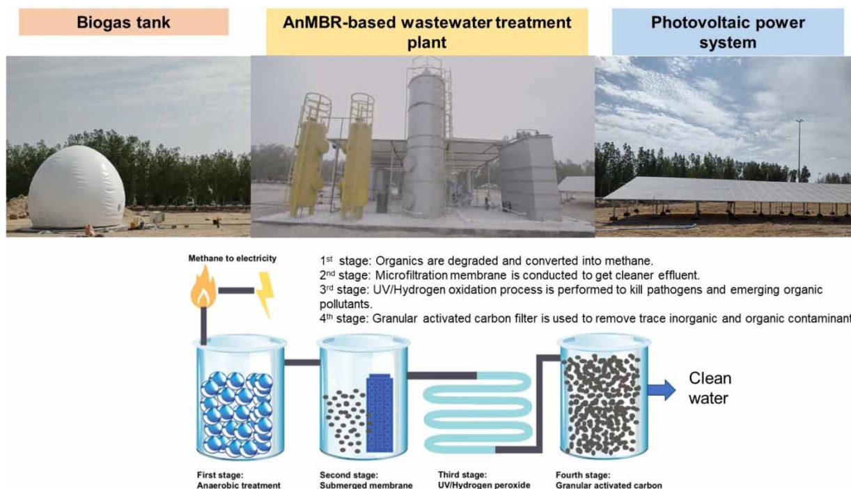
Figure 8 | A schematic representation of the demonstration-scale AnMBR-based wastewater treatment plant that is commissioned and currently under operation in Jeddah, Saudi Arabia. The treatment capacity for this plant is 50 m 3 /day and is entirely powered off-grid.
