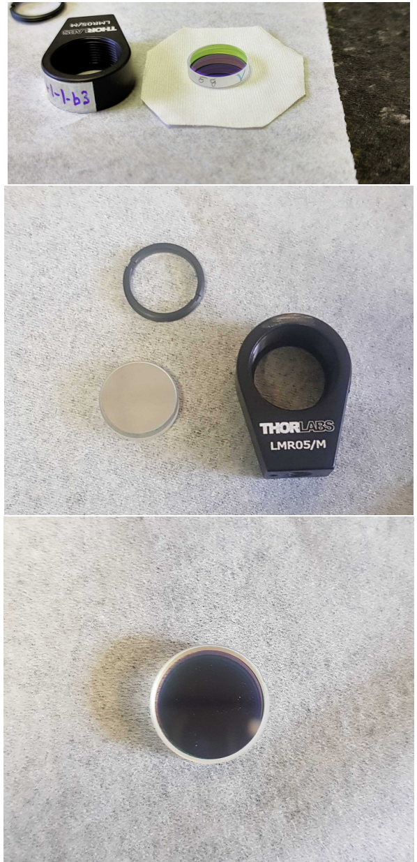
Figure 8: Top: Filter before first thermal cycle. Middle: The filter after the last cryogenic cycle showing no visible sign of wear. The Thorlabs LMR05/M shown in both pictures is the filter mount in which the dichroic D3 was mounted for cryogenic tests and optical characterisation. Bottom: Filter not mounted in the LMR05/M.
