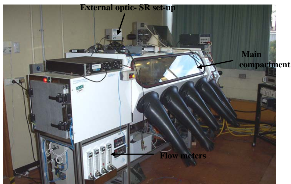
Figure 3.13. Glove Box used for electrical measurements (School of Mathematical and Physical Sciences, University of Newcastle, Australia).
