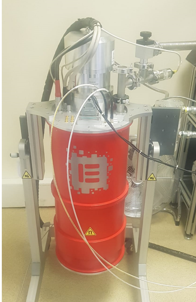
Figure 3.2: Entropy adiabatic demagnetization refrigerator (ADR) which is used to cool the MKID arrays down to below 100 mK using the magnetocaloric effect (MCE)
