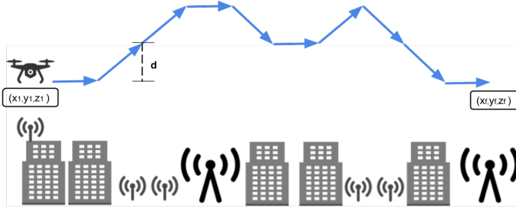
FIGURE 4.1: Side view of a UAV connected to the mobile network adjusting its height to maximise its throughput.
