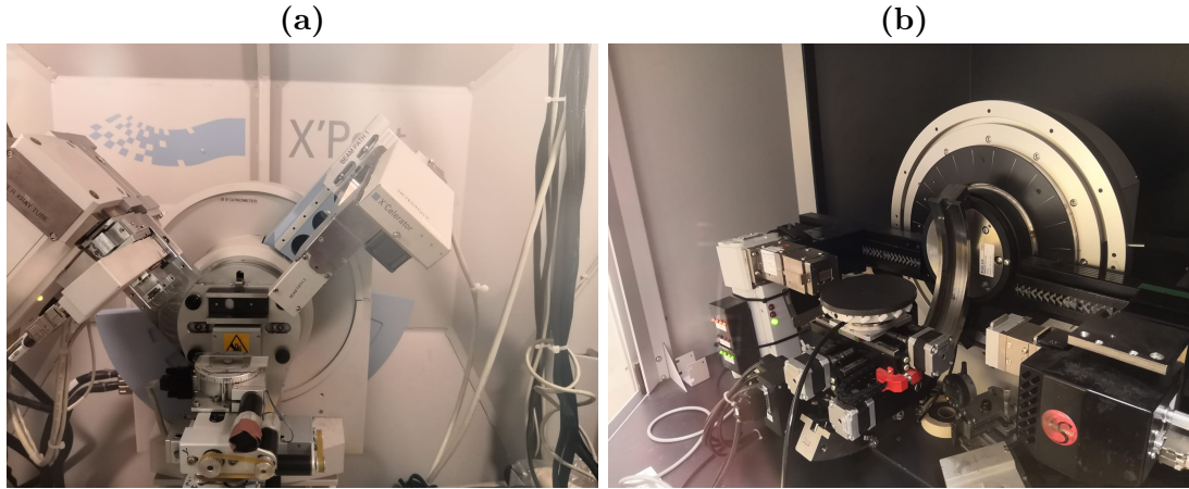
Figure 2.7: (a) Philips PANalytical X'Pert (PANalytical) X-ray diffractometer, (b) Bruker D8 Discover diffractometer (Bruker) X-ray diffractometers.
