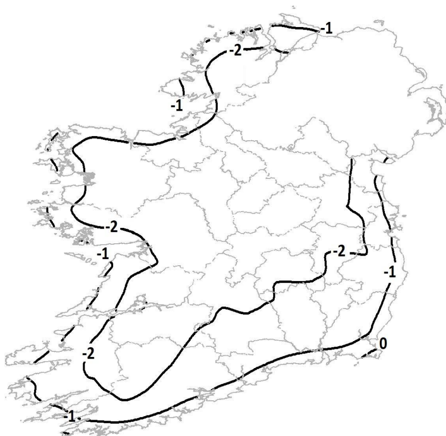
Figure 3: Isotherms of the lowest 10cm soil temperature (°C) for a 100-year return period in Ireland.
