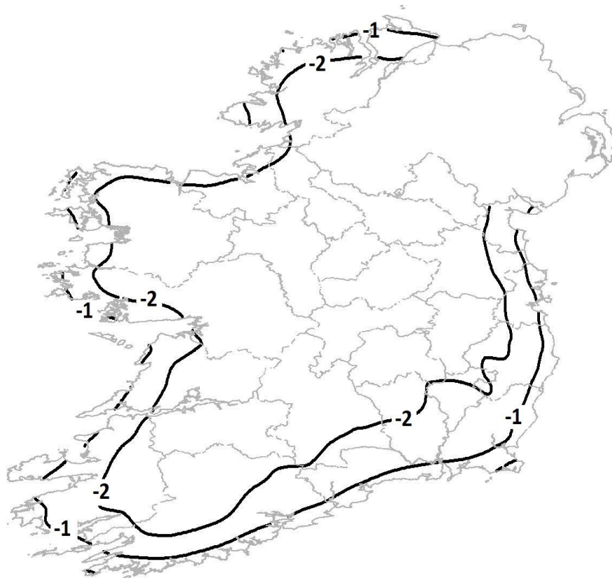
Figure 4: Isotherms of the lowest 10cm soil temperature (°C) for a 120-year return period in Ireland.
