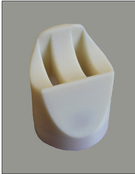
Figure 1. 3D printed section of hypothetical exoskeleton knee joint designed by David Taylor.
