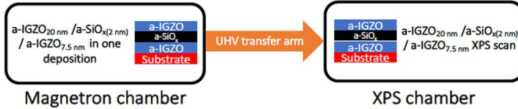
Figure 5.24: a\text{-IGZO}_{(20\text{ nm})}/\text{SiO}_{x(2\text{ nm})}/a\text{-IGZO}_{(7.5\text{ nm})} three-layer structure film was transferred with in-situ transfer of from magnetron to XPS under UHV transfer arm as shown in Figure 5.22.
