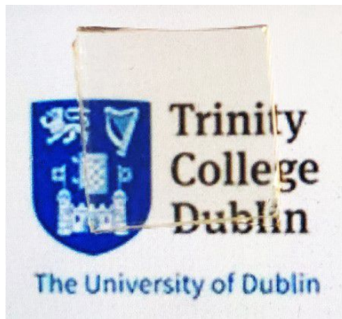
Figure 4.5: An image of 38 nm thick a-ZTO film deposited at 300^\circ\text{C} on Glass substrate.
