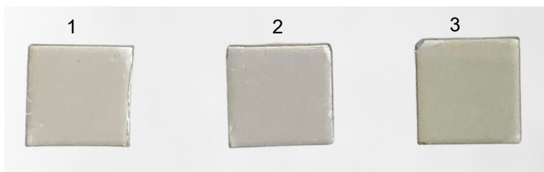
Figure 4.22: Images of a-ZTO films with different thicknesses, where (1) - 38 nm, (2) - 77 nm and (3) - 117 nm thick a-ZTO.
