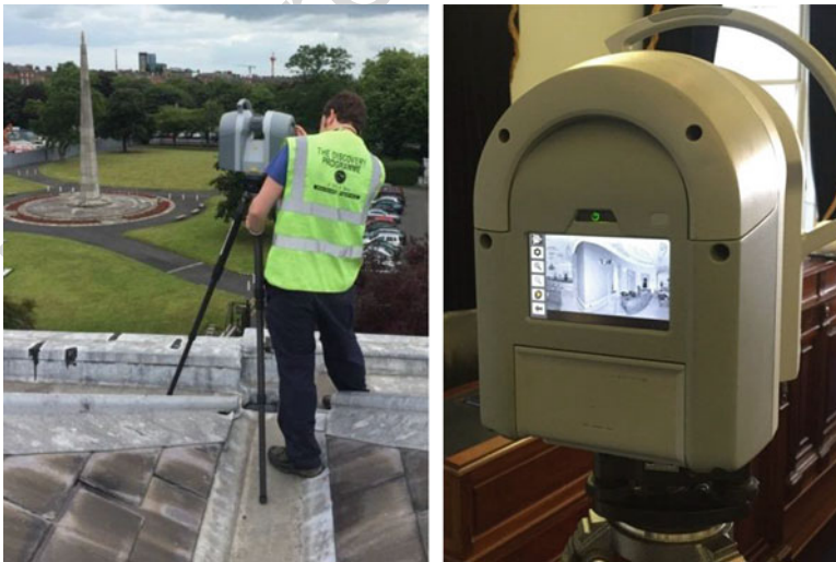
Fig. 51.2 Data capture, terrestrial laser scanner is a device that automatically measures the three-dimensional coordinates of a given region of an object's surface [2]
