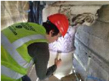
Fig. 51.3 For higher accuracy, the process of structured light scanning involves projecting a known light pattern onto the subject, Corinthian Capital Survey, Four Courts Dublin [2]
