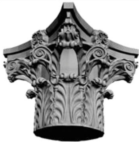
Fig. 51.3 For higher accuracy, the process of structured light scanning involves projecting a known light pattern onto the subject, Corinthian Capital Survey, Four Courts Dublin [2]
