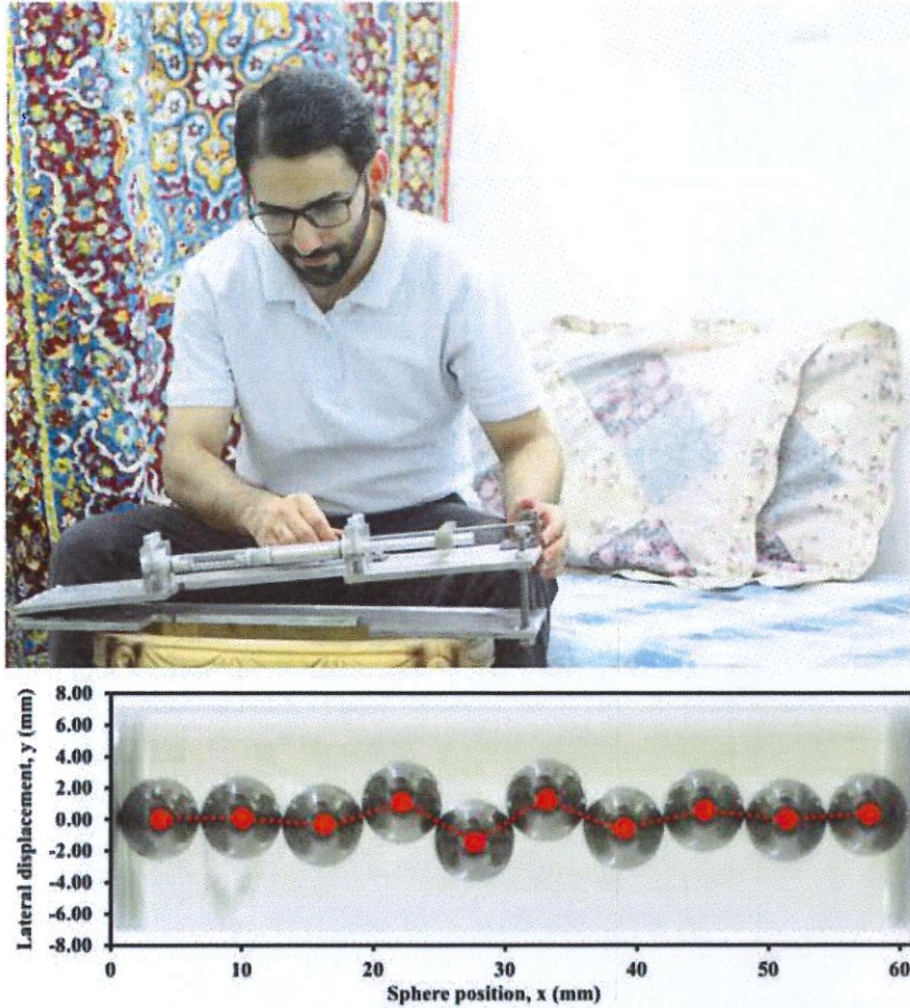
Fig. 1 One of the authors (AI) performing experiments in his bedroom in Tehran, Iran, during a Covid lock-down. His apparatus consists of a cylinder containing metal spheres. Pushing in the sides of the cylinder induces buckling of the initially linear chain. The effect becomes more and more localized as this compression is increased. In a variation of the experiment we study the position of the localisation peak as the cylinder is tilted, in order to determine the so-called Peierls-Nabarro potential [4]. This potential, originating in the theory of crystal dislocations, can tell us how the localized buckling moves when we tilt the apparatus. (This is difficult to investigate with hard spheres, easier with bubbles)
