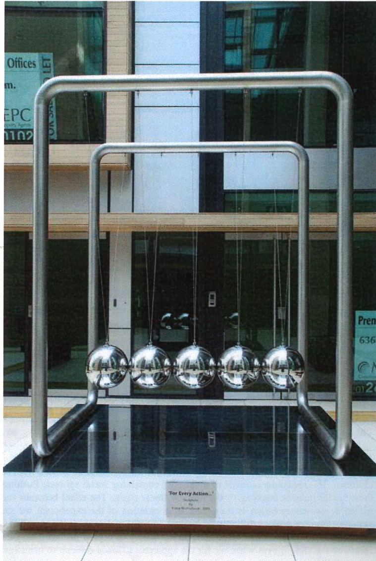
Fig. 2 In the standard textbook description of Newton's Cradle there is always only one sphere in motion. However, careful observation of the experiment shows that, already after the first impact of a displaced sphere on one side, the entire chain begins to break up, with all spheres in motion. Theory and computer simulations confirm this, and attribute it to the finite elastic modulus of the spheres [7]. The photograph shows the stainless-steel sculpture For every action ... by Fiona Mulholland (2005), permanently sited at Beacon Court South Quarter, Sandyford, Co Dublin. (Photo reproduced with kind permission by the artist)
