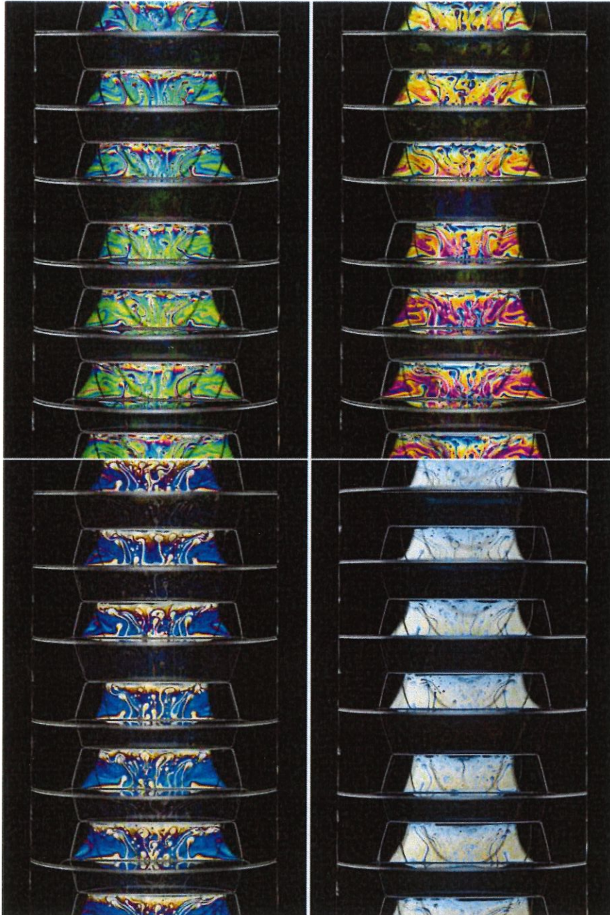
Fig. 6 Four photographs in a time sequence (top left to bottom right) of draining soap films in a “crystalline foam”, formed by soap bubbles, confined in a cylinder (©Kym Cox). The interference colours are indicative of the local thickness of the soap films. Since the foam structure is periodic in space, also the interference pattern seen in the films is repeated in each of the four photographs, with minor random fluctuations
