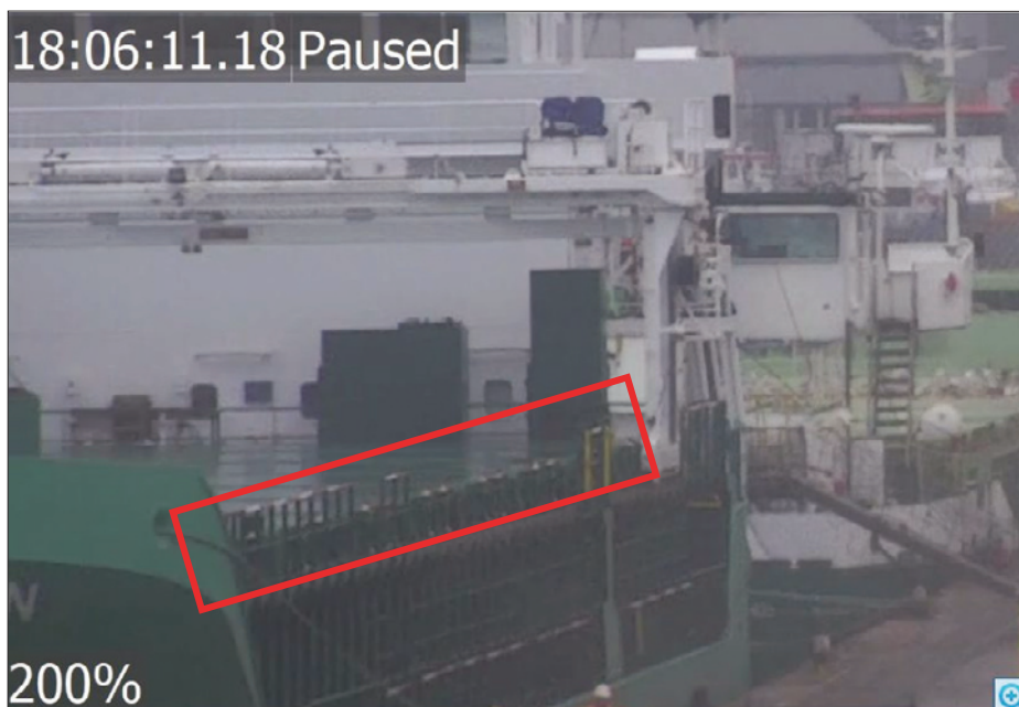
Photograph No. 3 - Position of Railings Post-fall. Partially in Down Position
