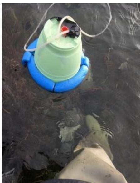
Figure 3.37. Modified flower pot for taking samples of air through the septum on the top of the pot.
