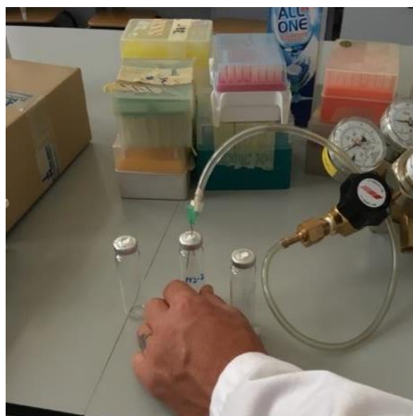
Figure 3.45. Filling of vials with standard gas mixtures.
