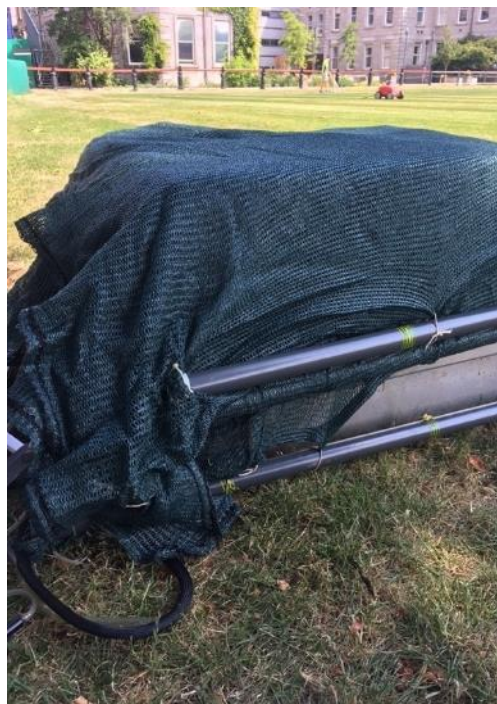
Figure 3.33. Chamber with covering to simulate shading.
