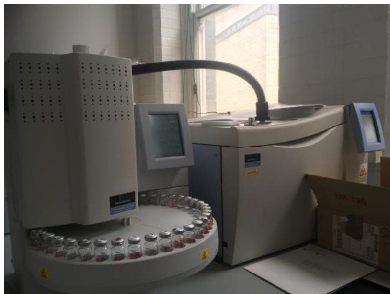
Figure 3.43. Perkin Elmer GC with autosampler.
