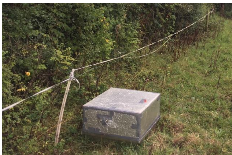
Figure 3.34. Opaque chamber for the measurement of CH 4 and N 2 O.
