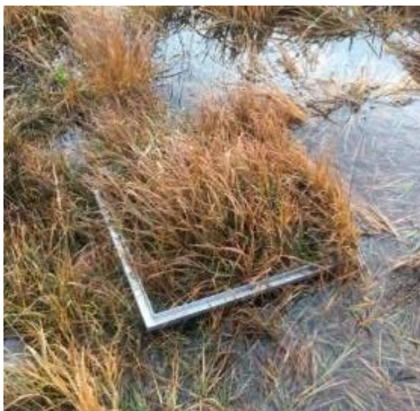
Figure 3.36. Metallic frame on flooded water (Measurements with transparent chamber and EGM4 infra-red device).
