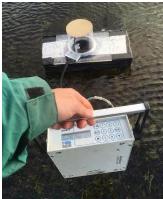
Figure 3.35. CPY-4 chamber connected to EGM-4 analyzer.
