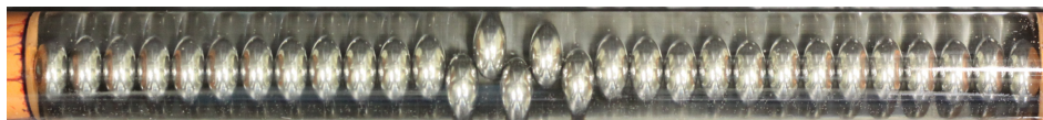
Fig 2.5: A chain of 30 hard spheres with a diameter of 6.32\text{ mm} confined in a perspex tube with an inner diameter of 1.6\text{ cm} is buckled under high compression illustrating a localized buckling. This represents one of the stable configurations and the situation can be symmetrical about the x-axis.
