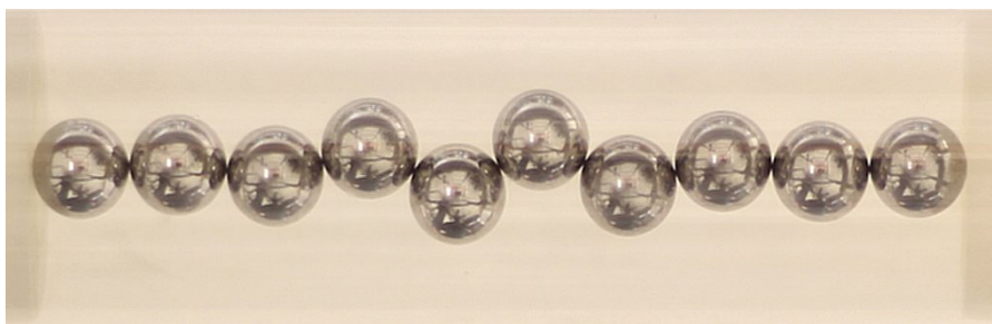
Fig 2.1: An example of a linear chain of 10 hard spheres (ball bearing) under compression which exhibits a zigzag pattern.
