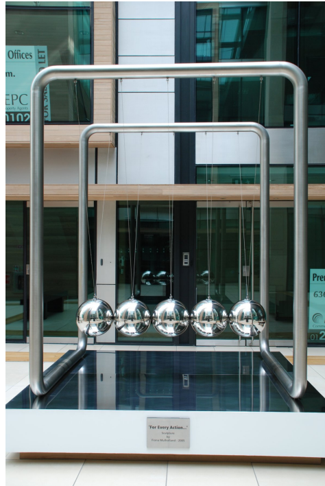
Fig 1.3: In the standard textbook description of Newton’s Cradle there is always only one sphere in motion. However, careful observation of the experiment shows that already after the first impact of a displaced sphere on one side, the entire chain begins to break up, with all spheres in motion. Theory and computer simulations confirm this and attribute it to the finite elastic modulus of the spheres [14]. The photograph shows the stainless-steel sculpture For every action ... by Fiona Mulholland (2005), permanently sited at Beacon Court South Quarter, Sandyford, Co Dublin. (Photo reproduced with kind permission by the artist).
