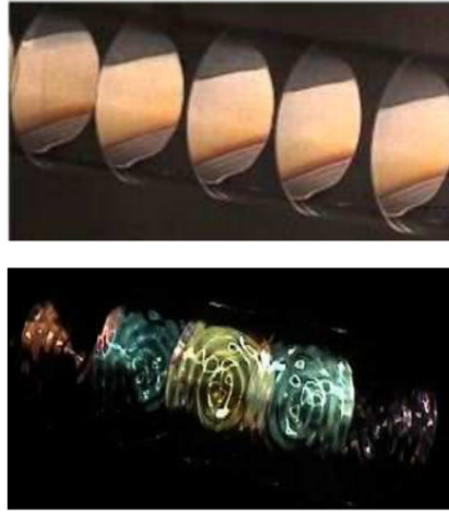
Fig 1.10: Visualization of sound waves using soap films. Top: Interference pattern in the absence of sound waves. The soap films are vertical and display a variation in colour (thickness) due to the gravitationally driven drainage Bottom: Fascinating patterns in the presence of sound waves. Measuring the distance between films with minimum interference patterns results in the wavelength of the sound wave.
