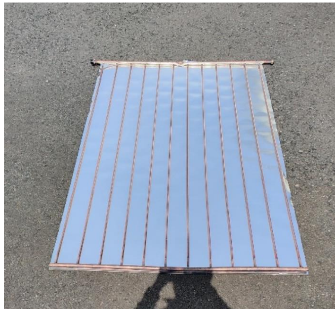
Figure 10. Dismantled solar thermal collector for individual component analysis
