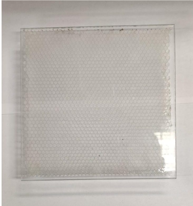
Figure 22. Overhead view of lab-scale model of the Novel Flat Plate Solar Collector (NFPC)
