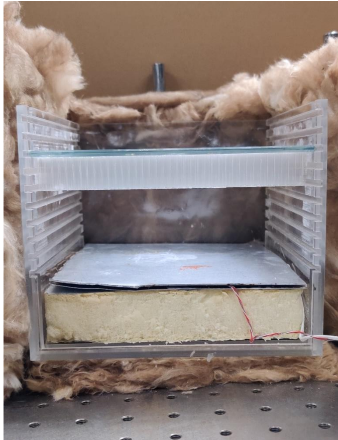
Figure 48. Experimental setup for the efficiency performance curve of solar thermal collector experiments
