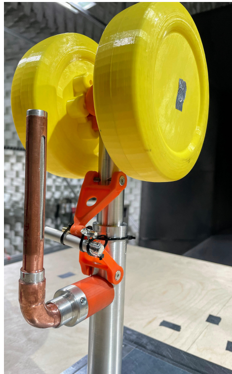
Figure 4.8: Modified torque-link air curtain with added rod for whistling sound
