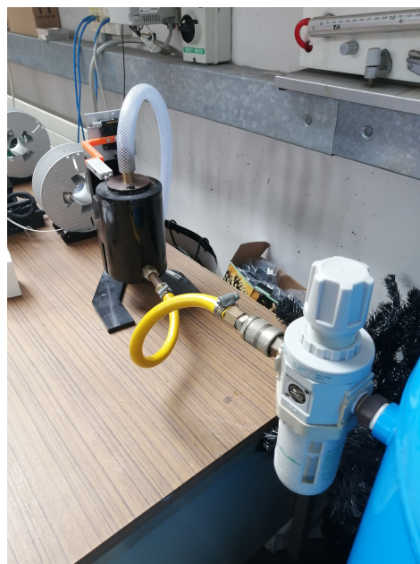
Figure A.4: Tank-to-chamber configuration during hot-wire anemometry tests
