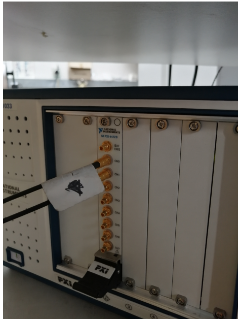
Figure A.11: Connections on the PXI-1033 controller
