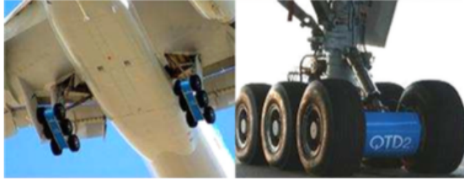
Figure 2.7: “Toboggan”-like fairing attached to the B777-300ER main landing gear in the QTD 2 Project [3]
