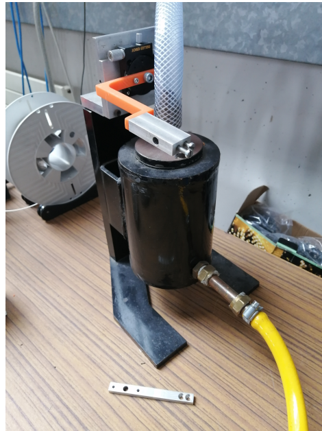
Figure A.5: Orange hot-wire probe holder or grey hot-wire probe holder to maintain the probe above the opening (grey hose to be removed for calibration)
