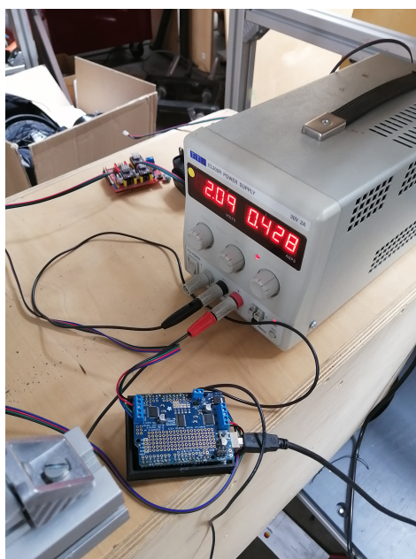
Figure A.8: Generator used to power the motors via the Arduino board
