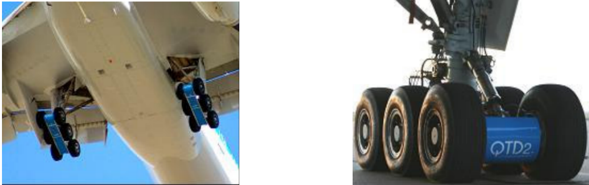
Figure 2.3: 'Toboggan' fairings attached to the main landing gear of the Boeing 777-300ER
