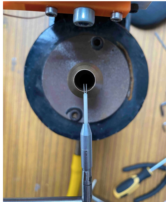
(b) The hot wire probe was placed at the outlet of the high velocity nozzle. It is important to note that it must be positioned with the same orientation as it will have for future velocity measurement tests.
