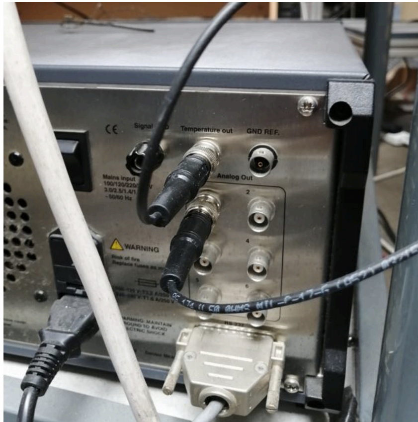
Figure A1.3: Rear view of StreamLine 90N10 frame with thermometer connection, probe connection to Analog Out 1, connection to PXI controller (silver) and power supply (black).
