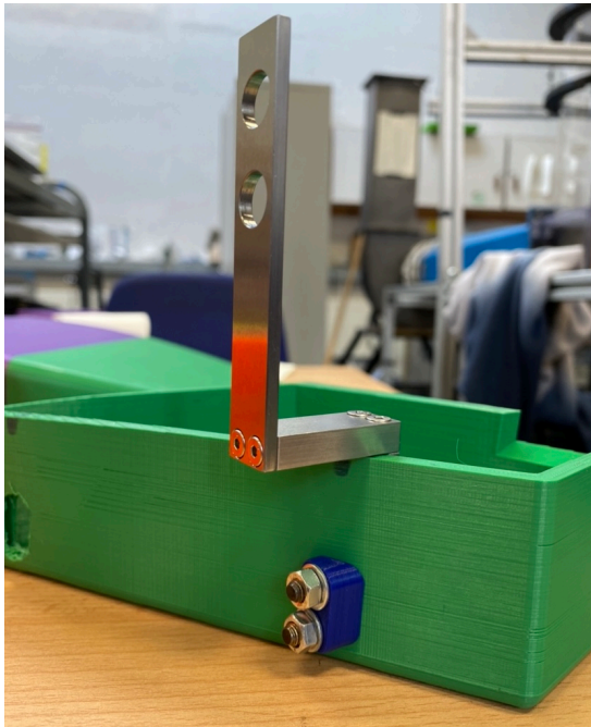
(a) The main leg (ML) bracket for the local nozzle is bolted on to the landing gear bay (green).
