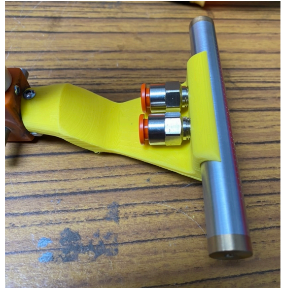
(b) The wheel bracket for local nozzles screws directly onto the landing gear.
