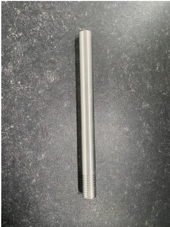
(a) Air tube design, featuring grooves on the open end to facilitate clamping of the air hose.
