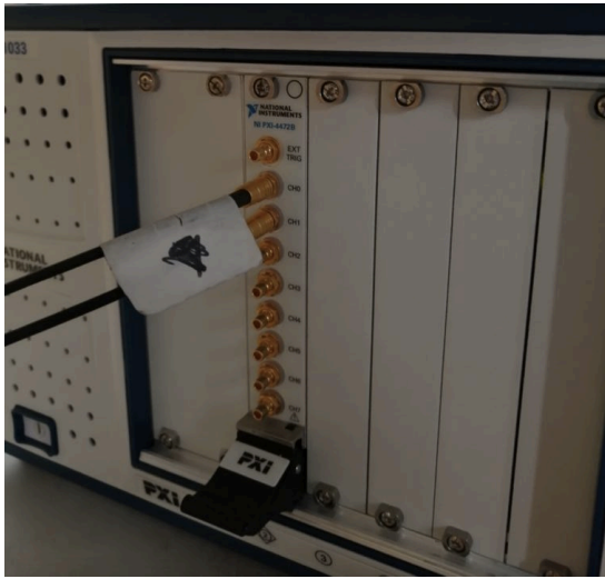
(a) PXI controller with hot wire probe connected to Ch0 and temperature probe connected to CH1
