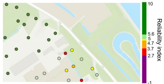
Figure 2 Exit point based piping assessments from the SAFE project. Colors indicate the safety of a point.
