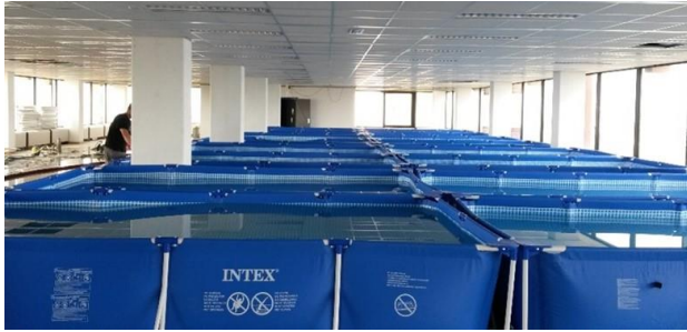
Figure 1: Load Test - Leopold II building
