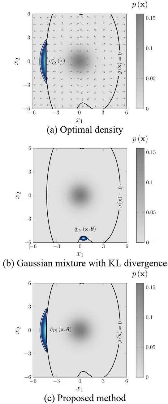
Figure 2: The contour plot of the importance sampling density for a metaball limit-state function.
