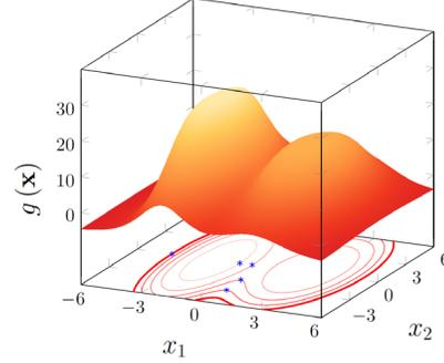
Figure 1: The limit-state function  $g(\mathbf{x})$  and design points (blue asterisks) on its level-sets (red curves).
