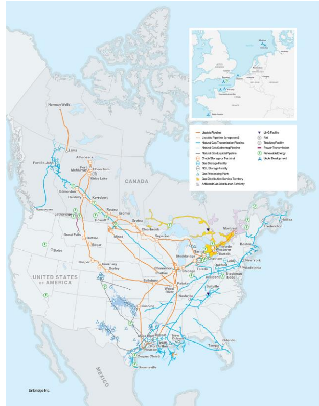
Figure 2: Geographical extent of the gas transmission pipeline system (shown in blue) in North America
