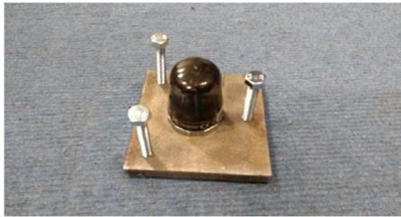
Figure 2: Lord sensor mounted on 8 mm steel plate and three adjustable bolts.
