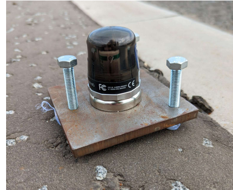
Figure 3: Lord sensor positioned near the top of kerbside before recording.
