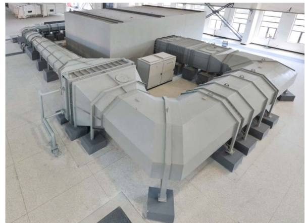
Fig. 1. FLY-17 0.55 m × 0.4 m aeroacoustic wind tunnel: (a) dimensions (mm); and (b) full view.
