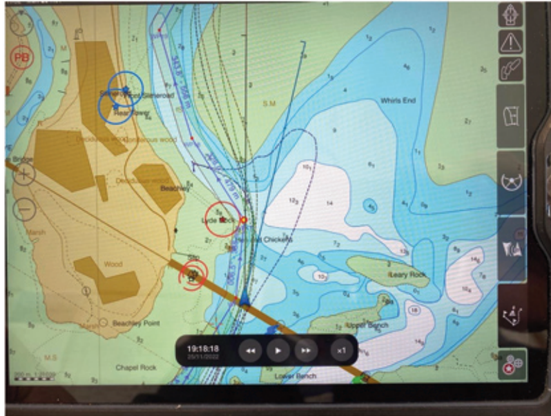
Fig.4: Screenshot of PPU showing inwards track to grounding, plus subsequent outwards track. Also tracks of prior vessels with same Pilot.
