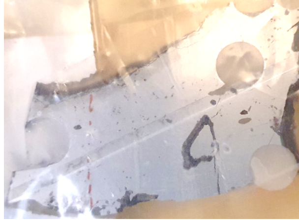
Figure 4.22: The polished sample from the meteorite. The circular indentations and other straight-edged marks are from cuts taken from this piece for other measurements before we obtained the sample.
