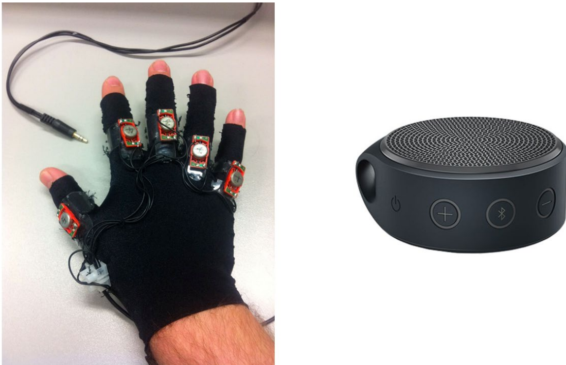
Figure 5. Vibrotactile devices ( left —audio-tactile glove; right —Logitech X100).
