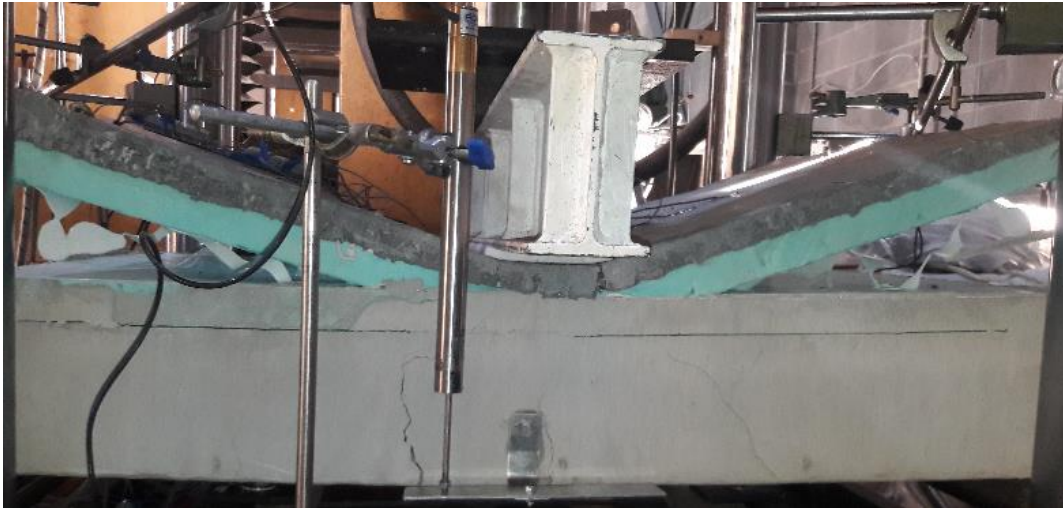
Figure 6-14 Control No Ties panel at ultimate failure showing deflection at end of panel and failure of the lower panel
