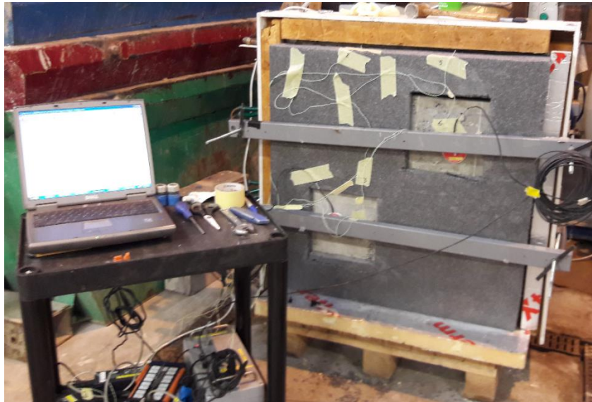
Figure 3-9 Photograph of thermal testing of sample panels
