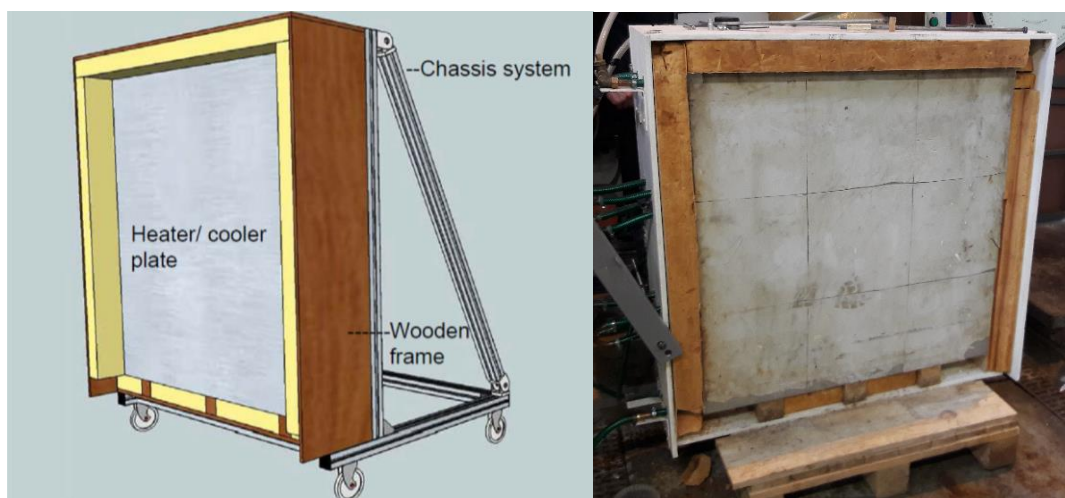
Figure 3-8 Schematic (Byrne et al., 2017) and photograph of adjusted hot plate apparatus
