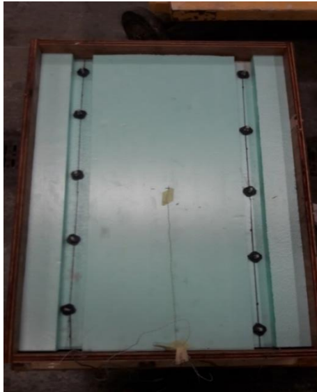
Figure 5-7 PCM-concrete panel with Thermomass connectors
