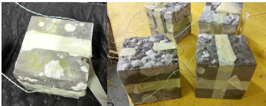
Figure 4-5 Mould-like substance on the surface of the concrete samples
