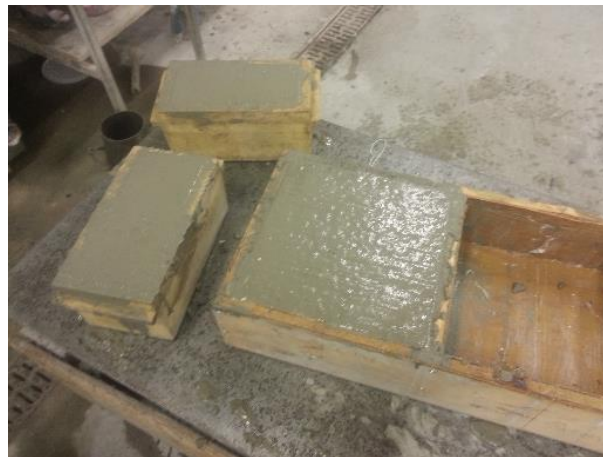
Figure 4-8 Photograph of trial control mix placed in the formwork
