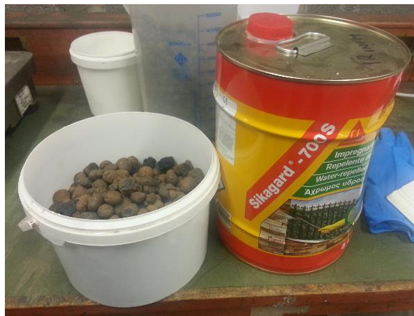
Figure 3-4 Image of LWA-PCM composite after sealing with Sikagard 700S
