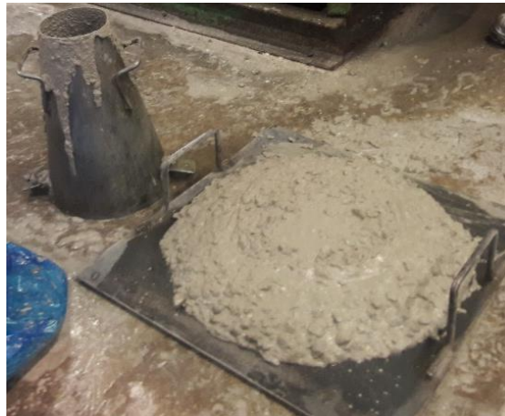
Figure 5-3 Slump flow test of the control mix concrete
