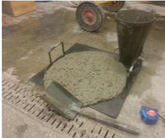
Figure 4-10 Photograph of trial PCM-concrete mix
