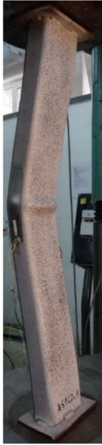
Figure 1.4: Examples are shown here of the first two modes of Euler buckling of the system shown in Figure 1.3 (reproduced from [20]), the first two solutions of Eqn (1.1). The variety of structures are characterised by the initial angle \theta(0) = \alpha . Note that the distance between the supported ends, d , is a function of this angle. A physical example of the first mode can be seen on the left, showing the buckling of a concrete-filled steel tube under compression (image reproduced from [21]).
