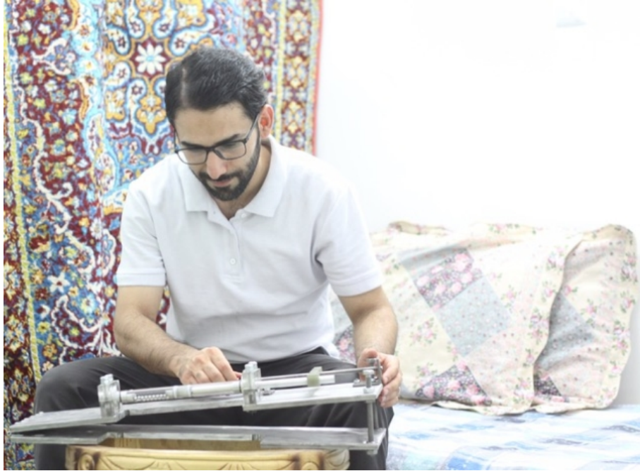
Figure 1.9: Ali Irannezhad and the experimental apparatus he had commissioned to study the buckling of a line of spheres under compression and tilt. This image was featured in an article titled 'Physics in a Small Bedroom', highlighting experiments that were rich in detail and yet could be carried out outside the lab (Image reproduced from [31]).
