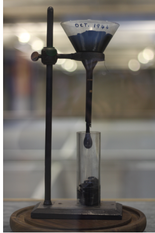
Figure A5.3: A photo of the Trinity College Dublin pitch drop experiment (image credit Jennifer Quirke). At time of writing the experimental apparatus is available to view in the Library, and the current drop would be expected to break off around 6 years from now.
