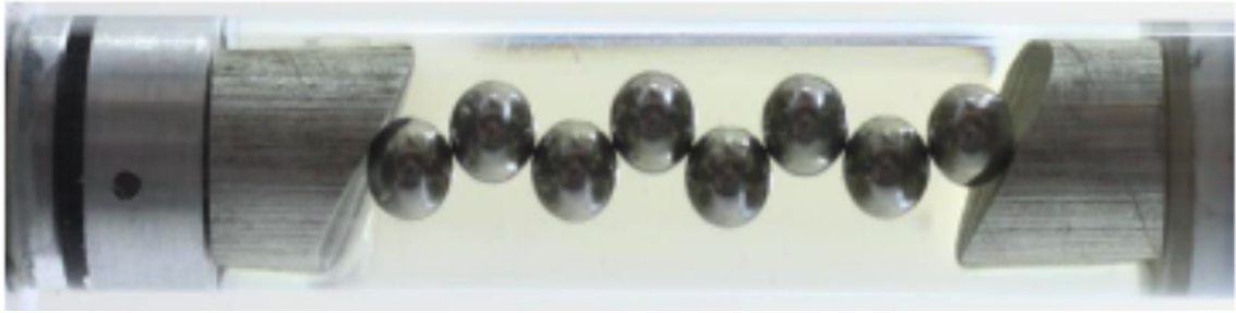
Figure 7.2: It is possible to vary the value of the boundary angle, \phi(0) , by modifying the experimental method detailed in Section 1.3. Here the originally straight boundaries are replaced with sloped stoppers, influencing a more uniform zig-zag profile. Although the stoppers pictured here are parallel, they do not necessarily need to be. Image credited to Ali Irannezhad.
