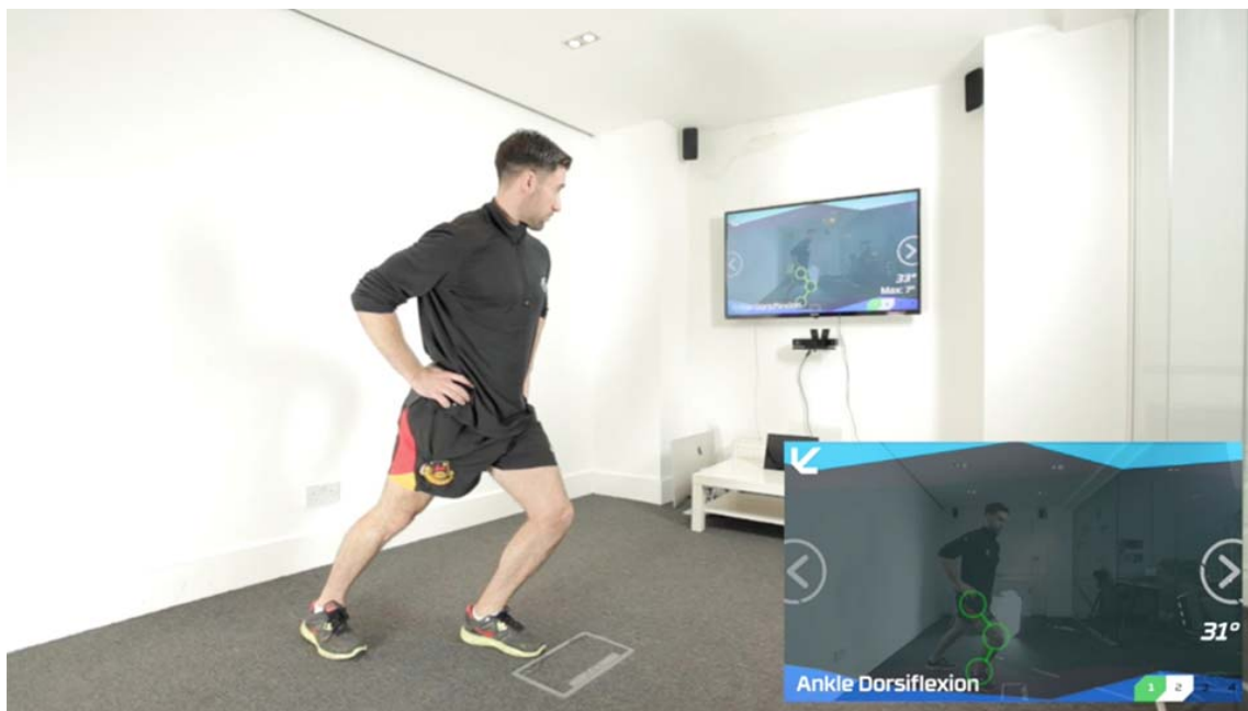
Figure 1: field test of CAPTURE during an ankle dorsiflexion measurement. The result displayed is the angle between the lower leg and a reference vector connecting the knee and the closest point on the floor.
