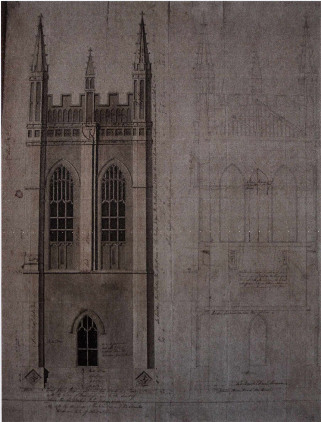
Fig. 2.1 Proposed elevation and section of a two-storey battlemented Gothic tower for St Patrick's Cathedral, Armagh (C of I), attrib. to Thomas Cooley, [1784], IAA, RIAI Murray Collection no. 92/46.75, courtesy of the Irish Architectural Archive.
