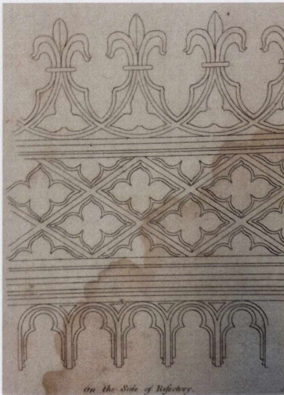
Fig. 3.21 'Rails, cornices and arched modillions', from Murphy, Plans, Elevations, Sections and Views of the Church of Batalha (1795).
