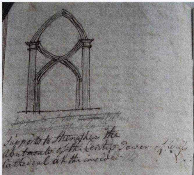
Fig. 1.20 'Supports to strengthen the abutments of the centre tower of Wells Cathedral at the inside', Laurence Parsons, 1786, Tour journal, f. 19v.
