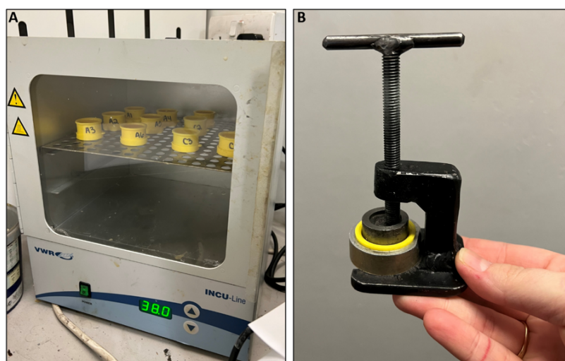
Figure 4.3. (A) Coral sample pucks hardening in oven and (B) “Puck-Off” device used to remove cured pucks from mount.
