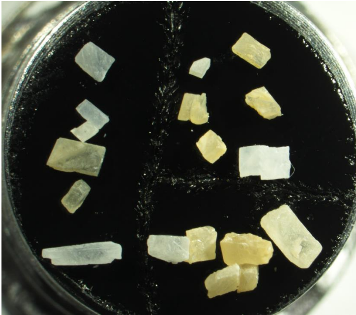
Figure B7.1: Calcite seeds post reaction with Sr-bearing solutions display (puck diameter 12 mm)
