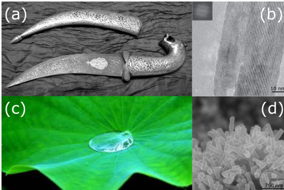
Figure 1.2: (a) Damascus steel blade. (b) TEM images depicting carbon nanotubes in Damascus steel. (c) Water droplet on Lotus leaf exhibiting hydrophobicity. (d) SEM image of Lotus leaf surface. 24-27
