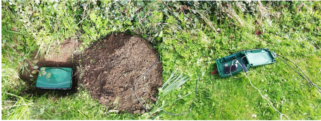
Figure 3.11: The magnetometer was buried about 50 cm down using waterproof junction boxes to house the magnetometer and data logger separately (right). The magnetometer was buried to reduce noise and help thermal stability.
