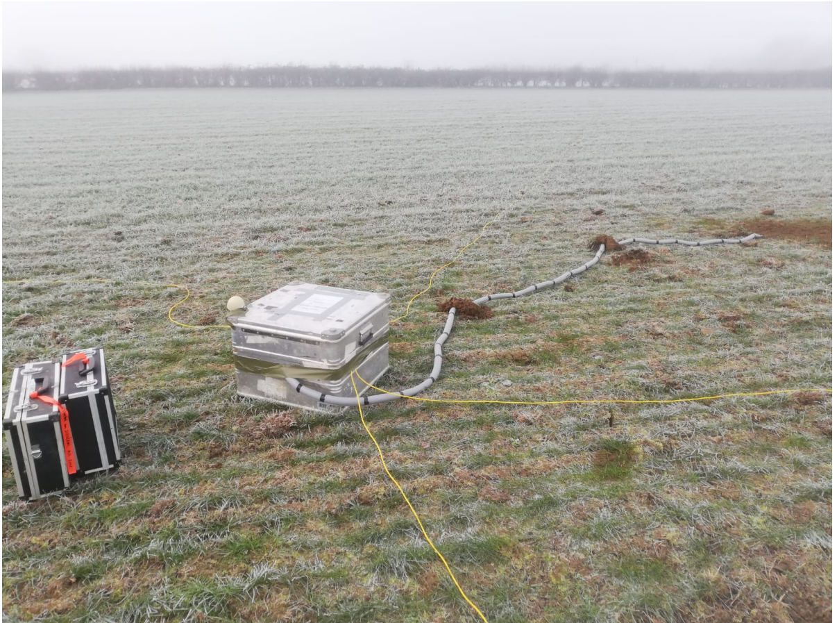
Figure 5.3: An MT site from the HI-RES survey. The data logger and battery are contained in the aluminium box (centre). The yellow wires extend out 40 m to the electrodes. The wire covered in foam insulation leads to the hole where the magnetometer is installed. The small pale-coloured orb on the other side of the aluminium box is the gps unit. The yellow wires were later buried at this specific site.
