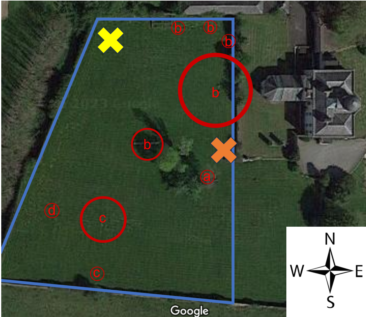
Figure 3.15: A map of the area considered for installation of the permanent magnetometer in Dunsink, denoted by the blue box. Magnetic anomalies recorded are marked roughly using red circles, roughly marking the area affected by the magnetic anomaly (to approximately 5 nT). Letters were used to denote the sources: a) red brick wall, b) buried/visible iron related to the walls, c) unknown, d) manhole lid. The buried location of the currently installed temporary magnetometer and planned for permanent are also highlighted by orange and yellow crosses respectively.
