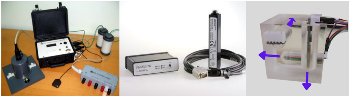
Figure 3.8: Each magnetometer brand is shown; the LEMI 417M magnetometer is on the left, the SENSYS FGM3D in the middle and raspberry pi on the right frame of the image. (left) The LEMI magnetometer is made up of the fluxgate on the left side, data logger in the middle, with the option to attach electrodes (the cylinders on the right side) for electric field measurements. (middle) The SENSYS logger is on the left and magnetometer on the right side. (right) The raspberry pi magnetometer is made up of the three FLC-100 magnetic sensors oriented inside a perspex block.
