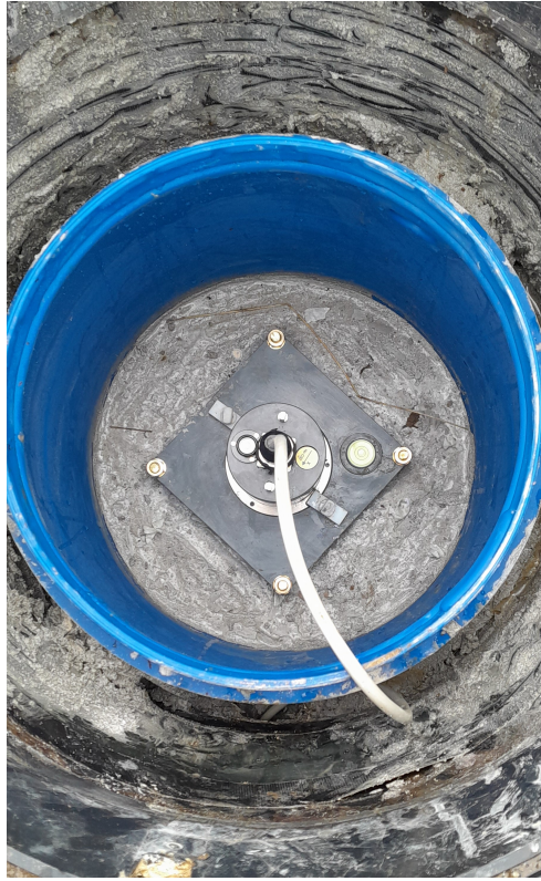
Figure 3.16: The repaired Birr magnetometer chamber. The new chamber (in blue) is placed in the old chamber (in black) with a new magnetometer base plate at the centre for mounting. Brass screws are used to make slight adjustments to the alignment of the plate.
