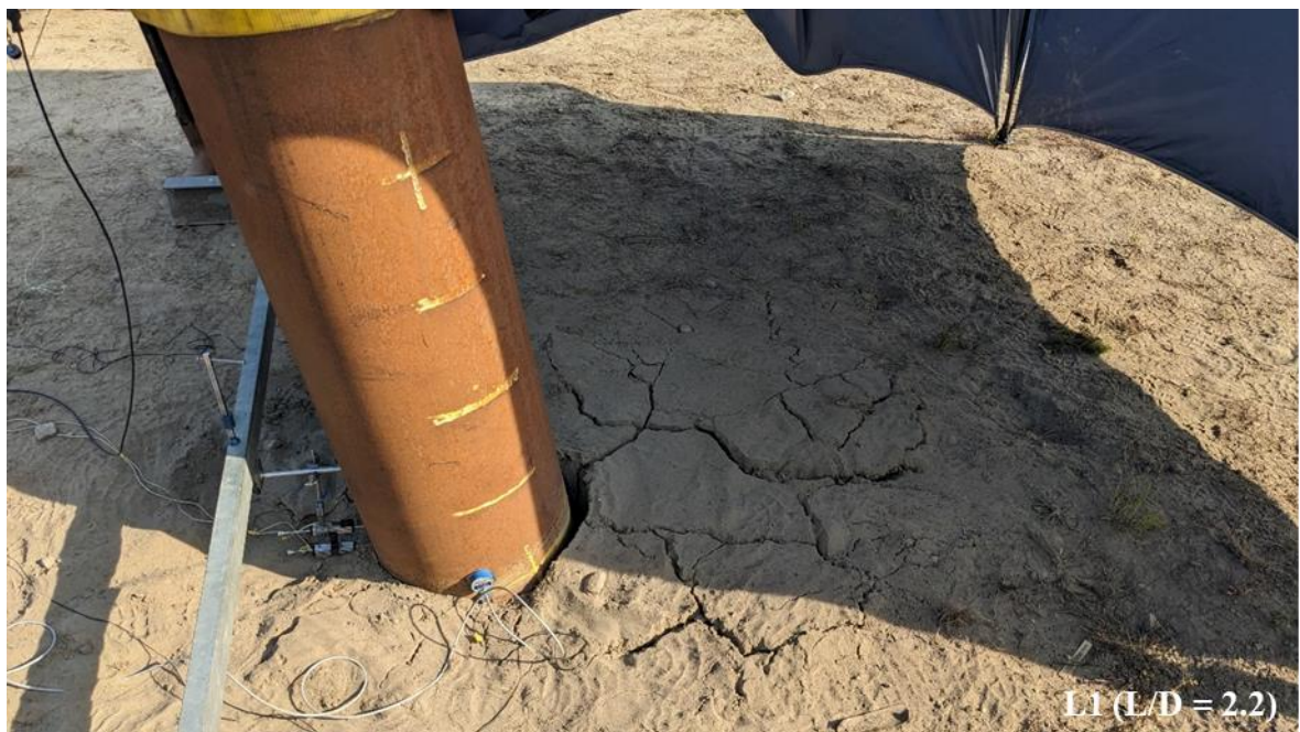
Figure 4-8. Example of gapping and soil cracks after completion of the cyclic tests for pile L1 ( L/D = 2.2 )
