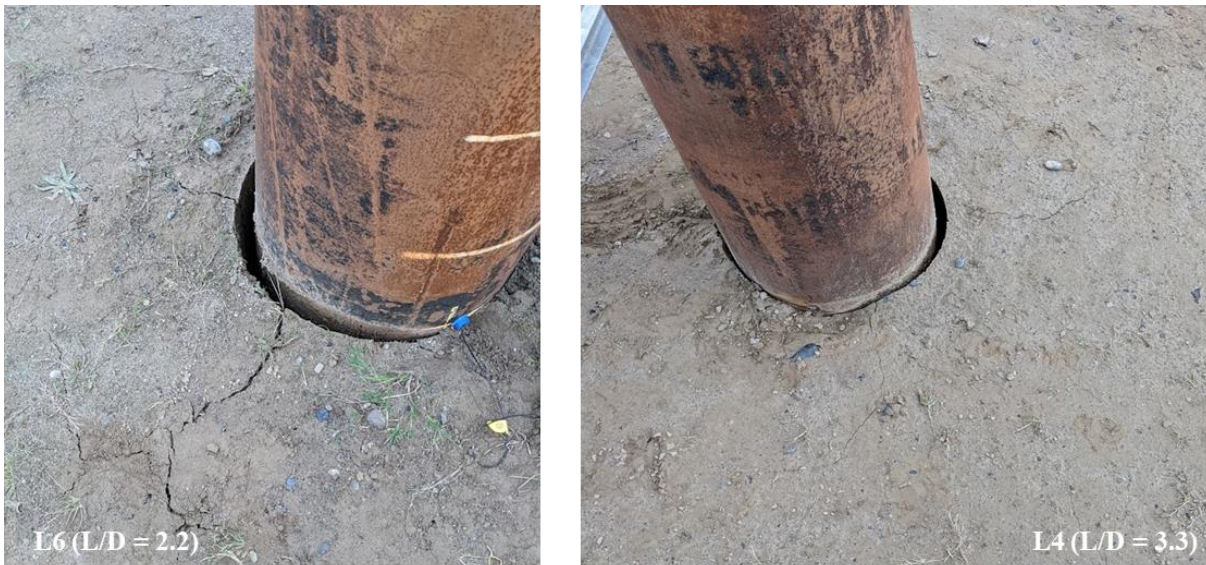
Figure 3-13. Example of gapping and soil cracks after completion of the monotonic tests for L6 ( L/D=2.2 ) and L4 ( L/D = 3.3 ).
