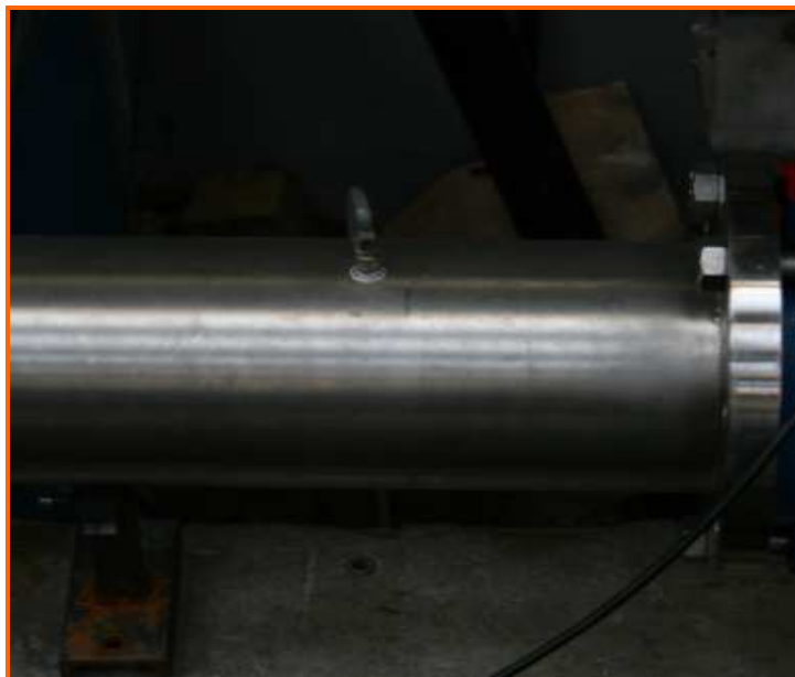
Figure 3.13 : The pressure tap at 1 D upstream from butterfly valve
