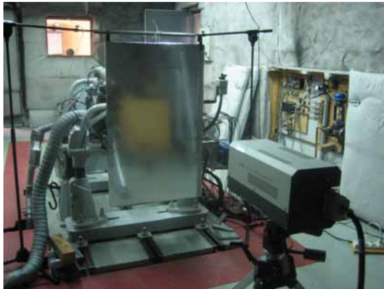
Fig 3.5 Rig of motor's noise measurement
