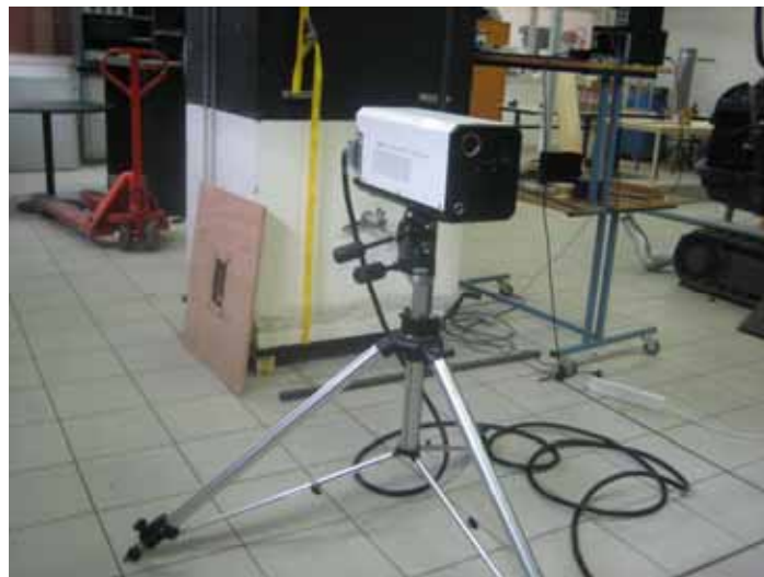
Figure 3.2 Polytec OFV 056 Vibrometer Scanning Head
