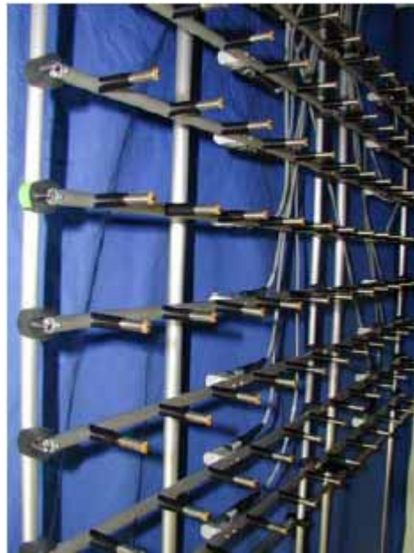
Figure 1.3 96 high-precision microphones combined on an array and connected to an analyzer. From [13]
