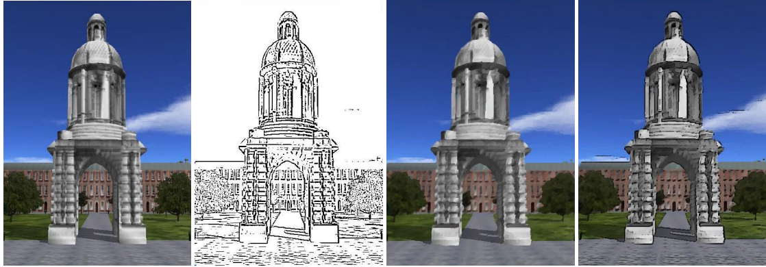
Figure 1: Example of various renderings of the same part of a scene. (a) A normal rendering with no abstraction (b) The edge image retrieved from Difference of Gaussian edge detection (c) Output image from the Kuwahara filter using 3x3 sampled regions (d) The edge image overlaid on the Kuwahara image.
