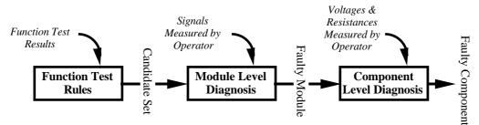
Figure 1. The main components in the NODAL fault diagnosis system.
