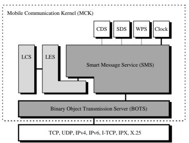
Figure 2. The structure of the MCK router is split into core services and support services. The CDS, SDS, and WPS are directory services which supports a 3-level routing hierarchy. The LES and LCS support an event system which delivers events to smart messages. These constitute the support services. The core services are the SMS and the BOTS servers. Note: our SMS server has no relationship to the Short Messaging Service in GSM. These directly implement the routing functions for smart messages.
