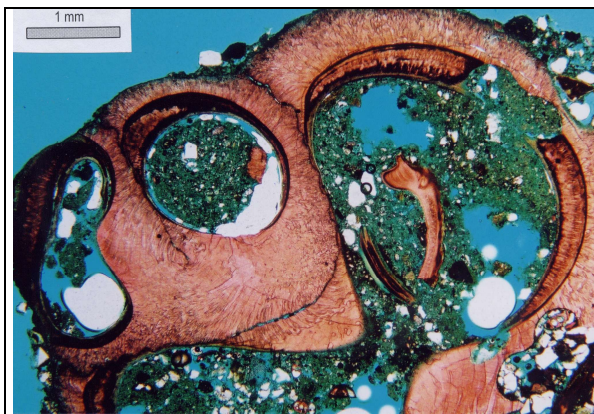
Figure 11. Cross sections of shells evidencing the use of beach sand in the lime mortar of Carrigafoyle Castle, Co. Kerry, Ireland. 2X, plane polars.
